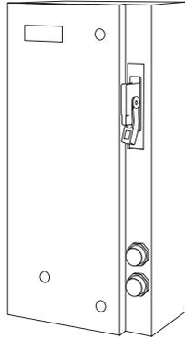
In many commercial and industrial applications quite a few electric motors are required, and it is often desirable to control some or all of the motors from a central location. The apparatus designed for this function is the motor control center (MCC). Motor control centers are simply physical groupings of combination starters in one assembly. A combination starter is a single enclosure containing the motor starter and the fuses or circuit breaker.
