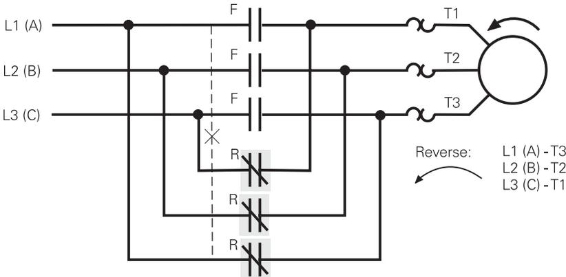
Many applications are designed for forward and reverse operation. An overhead crane, for example, might use the forward direction to raise the crane and reverse direction to lower the crane.
