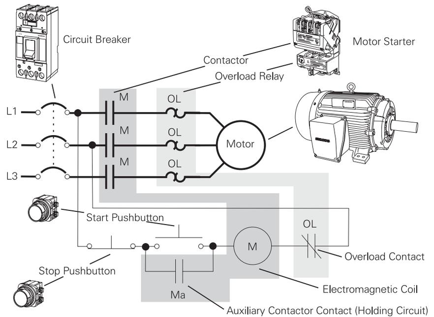
Typically one motor starter controls one motor. When only a few geographically dispersed AC motors are used, the circuit protection and control components may be located in a panel near the motor.
