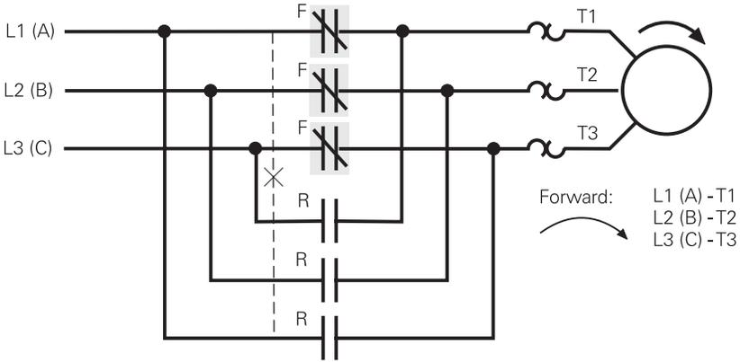
However, by reversing any two of the three power supply leads, the motor will run in the opposite direction. In this example L1 (A) is connected to motor lead T3, L2 (B) is connected to motor lead T2, and L3 (C) is connected to motor lead T1 (L1 and L3 have been reversed). When power is applied through the "R" contacts the motor will run in the counterclockwise, or reverse direction.
